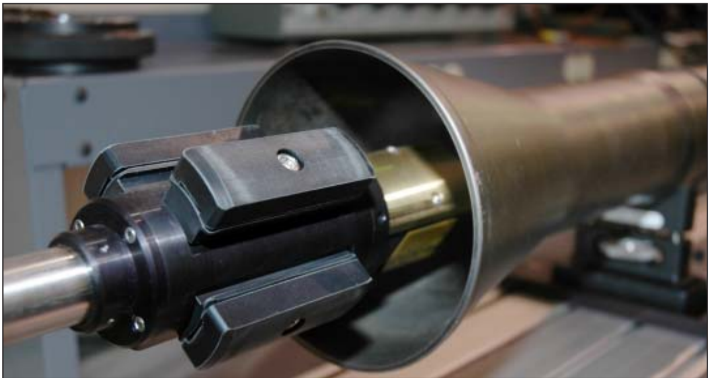
UP CLOSE AND PERSONAL – The laser-based bore mapping system scope prepares to enter a developmental 81 mm tube. The scope will send back three dimensional electronic data. (Photos by Public Affairs Staff)
